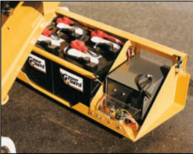
Swing-out compartment doors provide excellent access to hydraulic and electric components.
