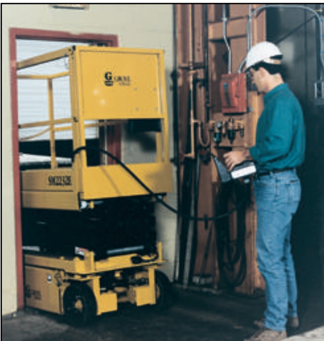
Compact dimensions allow access through standard doorways with rails installed.
