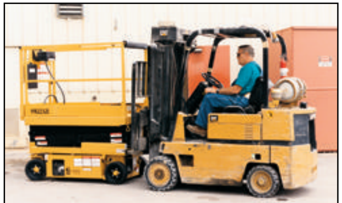
Fork lift pockets simplify loading and unloading and are ideal for transport around large job-sites.
