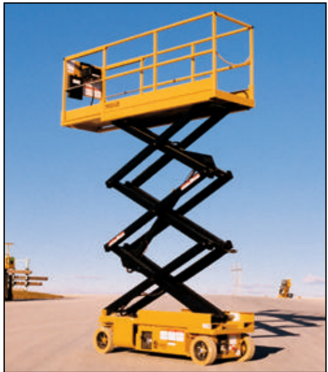
For reaching over obstacles, the SM2632E offers an optional 6 ft. (1.8 m) hydraulically operated deck extension with a capacity of 700 lbs. (317 kg). (Note: Unit cannot be driven with optional deck extended.)
